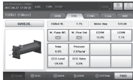
State of evaporator
